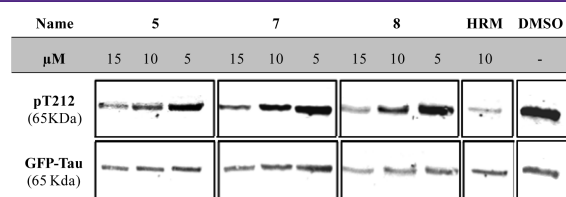
Figure 2. HEK293-tau-Dyrk1A cell assay. Compounds 5, 7, and 8 inhibit Dyrk1A-catalyzed tau phosphorylation in stably transfected HEK293 cells. The test compounds, DMSO, or the reference inhibitor harmine (HRM) 25,26 were added to the cell medium at the indicated concentrations. After immunoblotting, the level of phospho-tau-Thr212 was detected using a phosphospecific antibody. To normalize the signals, total recombinant tau protein was quantified using an anti-GFP antibody. One representative experiment out of two is shown.
